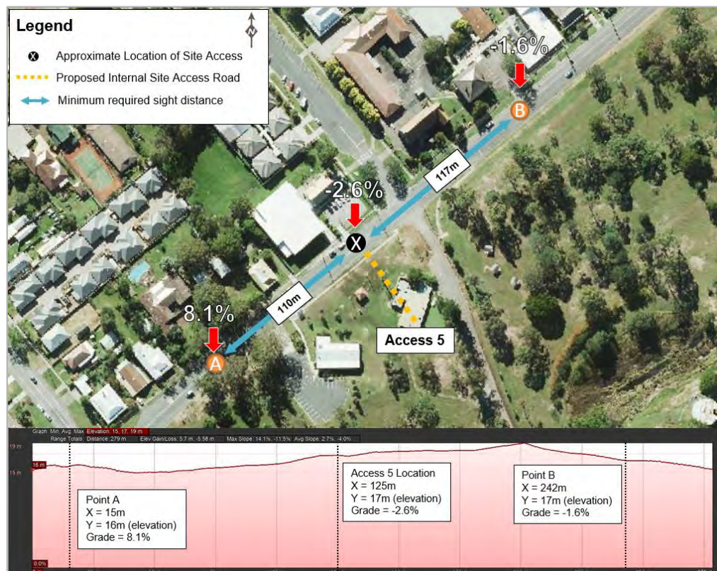
Figure 7-31 Access 5 – sight distances and longitudinal grades
